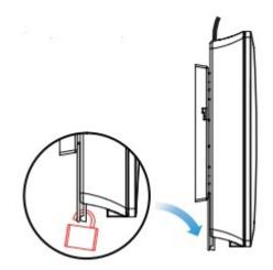
2) If the AP is installed on the wall, hold the AP in your hands and push it upward and away from the bracket in the LAN port direction.
